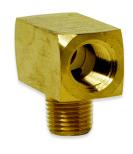
The BC Series are miniature Brass pipe fittings with various configurations of 10-32 inch UNF and 1/4-28 inch UNF male and female threads. These block fittings can be either female-to-female or male-tofemale configurations of elbows, crosses, or tees.
