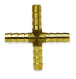
This series of Brass connectors is composed of straight connectors, elbows, tees, and crosses. The working temperature range is  $-40^{\circ}$  F to  $160^{\circ}$  F. The straights, tees, and crosses have equal barb sizes. The elbows are both equal and reducing. These fittings are designed for use with hose clamps.
