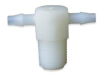
The AT-I Series is a Tee Adapter. These Tees can be made of Natural Nylon or Natural Polypropylene. It has 1/8 inch male NPT threads with barb sizes of 1/16 inch, 1/8 inch, and 1/4 inch. Also available in 10-32 UNF threads.
