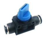
The HV Series Hand Valves are made with a PBT body, nickel-plated threads, and Buna-N O-rings. In addition, the valves can stop or reduce flow. The working pressure is 150 psi and the temperature range is  $32^{\circ}$  F to  $140^{\circ}$  F. They can be used for compressed air or inert gases.
