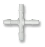
The CNRX Series is an equal single barbed Cross fitting. These crosses are available in Natural Nylon, Natural Polypropylene, and White Polypropylene. Available barb sizes are 1/8 inch and 1/4 inch.
