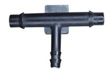
The VC-T Series is a series of single-barbed vacuum Tees, available materials are Natural Nylon and Red Nylon. Reducing Tees (VC-TR) are available in Natural, White, and Black Nylon 6/6. The temperature range for these tees is -20° F to 212° F. They can be used for air, liquid, and vapor.
