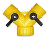
The 5114NS Series is a Garden Hose non-swiveling dual shutoff that has a non-corrosive plastic body, ball, and handle. Also, it has a Zinc plated steel screw and Buna-N seal. It flows from female to male. In addition, shutoffs are designed for city water pressure to a maximum of 80 psi. Furthermore, this valve does not swivel.
