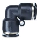
The PUE Series is a composite Union Elbow made of a PBT body and a Buna-N seal. The working pressure is 150 psi and a temperature range of  $32^{\circ}$  F to  $140^{\circ}$  F.
