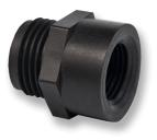
The MGHF Series is a Male garden hose by Female NPT threads garden hose fitting. Available FNPT thread sizes are 1/4 inch, 1/2 inch, and 3/4 inch. These fittings are available in either Nylon or Black Polypropylene.
