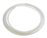
The SM Series is a medical-grade Silicone tubing that has been platinum-cured. It is resilient, stretchable, and resistant to compression. Also, it is UV, ozone, gas, and moisture resistant. This tubing is autoclavable with a durometer hardness of 50. Furthermore, its temperature range is -100° F to 500° F, meets FDA standards, and is NSF 51 listed.
