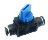
These Hand Valves are made with a PBT body, nickel-plated threads, and Buna-N O-rings. The valves can stop or reduce flow. The working pressure is 150 psi and the temperature range is 32° F to 140° F. They can be used for compressed air or inert gases.
