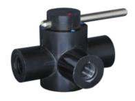
These ball valves are made of FDA Polypropylene with Viton® O-rings and 316 stainless steel handles. All connections are female NPT threaded. In addition, the pressure rating is 150 psi at 73°F. They are designed for use with liquid, gas, and vacuum applications. Inlet and outlet sizes are 1/8", 1/4", 3/8", 1/2", and 3/4". Also available in PVDF with actuation. Also, they are available in 2-way, 4-position 3-way, and 2-position 3-way orientations.
