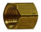
The BHFC Series is a Brass Cap that has female NPT threads. The working pressure is 1200 psi and the temperature range is -65 $^{\circ}$  F to 250 $^{\circ}$  F.
