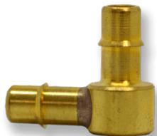
The BE Series Brass 90° Elbow bite-style connectors are fabricated with silver solder that complies with FDA, NSF, and medical grades VT lead-free and cadmium-free solder. Also available in 303 Stainless Steel. Included with the BE series is the BER series, which is the reduced version of the BE series.
