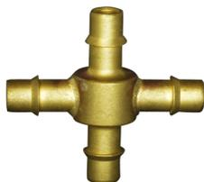
The BCX and the BCXR Series are bite-style cross fittings. The BCXR Series is the reduced version of the BCX Series. These crosses have single sharp barbs to securely hold the tubing from slipping or pulling off. They are excellent fittings for use with Polyurethane or Polyethylene tubing. Made in Brass, Nickel-Plated Brass, or 303 Stainless Steel. Available barb sizes range from 1/16 inch to 3/8 inch.
