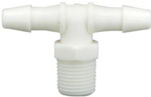
AT-S Series is an Adapter Tee available in black and white Nylon, black Polypropylene, and PVDF. There is straight male 10-32 UNF threads, male 1/8" NPT threads, and tapered 10-32 UNF threads. The barb sizes are 1/16" 3/32", 1/8", 3/16", and 1/4".
