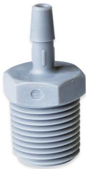
The A-R Series is a standard single barbed adapter. Available materials are Natural, White, and Black Nylon, Natural and White Polypropylene, Natural and Gray PVDF, Black Glass-Filled Nylon, and NSF 51/61 certified High-Density Polyethylene. Some sizes have Acetal and Black High-Density Polyethylene available as well. MNPT and barb sizes range from 1/8 inch to 1 inch. Male NPT threads are standard, but BSPT threads are available.
