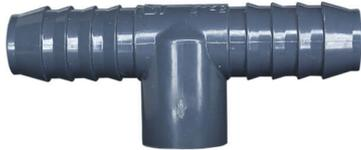
The SFT Series Tee adapter is made of PVC and can be used for irrigation and O.E.M. applications. There is a wide variety of configurations available for use with Polyethylene pipe sizes 1/2 inch through 2 inch. It conforms to ASTM D 2609 and is NSF-certified for use with potable water. Female NPT thread sizes are 1/2 inch, 3/4 inch, 1 inch, 1-1/4 inch, 1-1/2 inch, and 2 inch. Barb sizes range from 1/2 inch to 1-1/2 inch.
