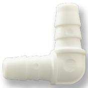
The L-IG Series are multi-barbed elbows made of Black and White Nylon and Gray Polypropylene. The ports are 1/16 inch and 1/8 inch. The maximum working pressure is 125 psi and the temperature ranges are: Nylon -50° F to 180° F; Polypropylene -40° F to 200° F.
