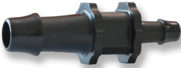
The C-U series is the ultimate high-flow single barb fitting for soft plastic tubing. The barb will expand the tubing up to 40%. This series is available as an equal or reducing fitting. Sizes ranging from 1/16 inch to 1 inch are available. Optional materials include Natural Nylon, Black Nylon, White Nylon, Polycarbonate, Polypropylene, and PVDF.
