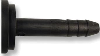
The FHS-B Series is a Plastic Multi-Barbed Hose Adapter Insert made of Black Polypropylene designed with a blunt end and extra long stem in sizes of 1/4 inch, 3/8 inch, 1/2 inch, 5/8 inch, and 3/4 inch. For use with 3/4 inch [FPN Series](#) Nut.
