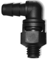
The ALS-IG Series Swivel Adapter Elbow allows tubing to be rotated 360° into position without crimping. These Swivel Elbows are made of Black Nylon. The male threads are 10-32 inch UNF or 1/8 inch and 1/4 inch male NPT. The barb sizes are 1/16 inch, 3/32 inch, and 1/8 inch. The 10-32 inch UNF threads are self-sealing, and the 1/8 inch and 1/4 inch threads seal with a Buna-N, EPDM, or Viton® O-Ring. The working pressure is 125 psi and the working temperature range is -50° F to 180° F.
