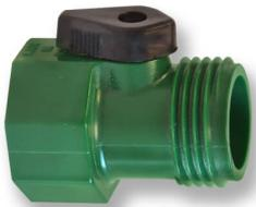
Single garden hose shutoff has an ABS body, ball, and handle. It has a Zinc plated steel screw and Buna-N seal. It flows from female to male. Maximum pressure is 80 psi, designed for water pressure. Maximum temperature is 125° F. Available in blue, green, or yellow.
