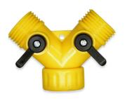
The 5114NS Series is a Garden Hose non-swiveling dual shutoff that has a non-corrosive plastic body, ball, and handle. Also, it has a Zinc plated steel screw and Buna-N seal. It flows from female to male. In addition, shutoffs are designed for city water pressure to a maximum of 80 psi. Furthermore, this valve does not swivel.
