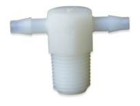
The AT-I Series is a Tee Adapter. These Tees can be made of Natural Nylon or Natural Polypropylene. It has 1/8 inch male NPT threads with barb sizes of 1/16 inch, 1/8 inch, and 1/4 inch. Also available in 10-32 UNF threads.
