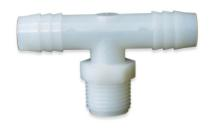
Male NPT thread by multi-barbed Tee Adapter is available in NSF-listed natural and black Nylon, NSF-listed black Polyethylene, and natural and black Polypropylene – both FDA-listed. Male NPT thread sizes are 1/8", 1/4", 3/8", 1/2", 3/4" and 1". The barb sizes available are 1/4", 3/8", 1/2", 3/4", 5/8" and 1".
