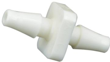
The C-SO Series are original single barbed straight and reducing connectors. These connectors have no parting line on the barb and have a square center hub. Also, tubing can be started on the barb of this connector before any expansion begins. It will expand the tubing by 43% when it is completely inserted. Available materials are Black and White Nylon, Natural Polypropylene, Clear Polycarbonate, and Natural PVDF. Available barb sizes are 1/16 inch, 3/32 inch, and 1/8 inch.
