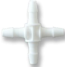
The CX Series is a standard single barbed Cross fitting with no molded parting line on the barb. The barb will expand the tubing to 50% above its normal size. It is available in White Nylon and Natural Polypropylene. The available equal barb sizes are 1/16 inch, 3/32 inch, and 1/8 inch. This cross-fitting is recommended for medical and laboratory environments.
