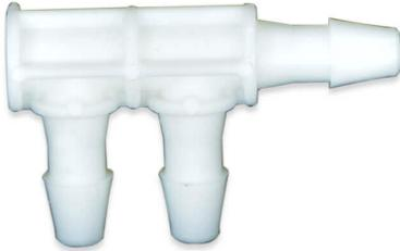
The DTF-S Series is a three-port F-style fitting usually used with flexible tubing. It can expand tubing by 50% of its normal ID. This permits high-pressure capabilities. This fitting is available in White Nylon and Natural Polypropylene. All three ports are equal. Available barb sizes are 1/16 inch, 3/32 inch, and 1/8 inch.
