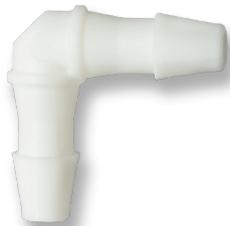
The EV Series are single barbed tube-to-tube elbows. These elbows are available in White and Black Nylon, Natural Polypropylene, Clear Polycarbonate, and PVDF. These elbows are available in equal or reduced sizes. Barb sizes are 1/16 inch, 1/8 inch, and 3/32 inch.
