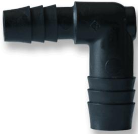
The L Series are standard triple-barbed elbow connectors and are offered in both equal and reducing sizes. These elbow connectors are molded of Natural Nylon or Polyethylene. Optional materials include: Natural and Black Polypropylene. Equal sizes are 1/4 inch, 5/16 inch, 3/8 inch, 1/2 inch, 5/8 inch, 3/4 inch, 1 inch, 1-1/4 inch, and 1-1/2 inch. Reducing sizes are 1/2 inch by 1/4 inch and 1/2 inch by 3/8 inch. Barbed fittings over 1 inch are not offered in Polyethylene.
