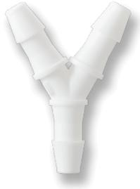
Y-S Series Wye tube fitting has equal single barbs and works well with flexible tubing. The barbs can expand tubing up to 50% above its normal size. This allows higher pressure capabilities. Available materials are White and Black Nylon, Natural Polypropylene, Polycarbonate, and PVDF. Barb sizes are 1/16 inch, 3/32 inch, 1/8 inch, 5/32 inch, 3/16 inch, and 1/4 inch. These Wyes are used primarily in laboratory and medical environments.
