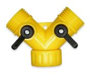
The 5114NS Series is a Garden Hose non-swiveling dual shutoff that has a non-corrosive plastic body, ball, and handle. Also, it has a Zinc plated steel screw and Buna-N seal. It flows from female to male. In addition, shutoffs are designed for city water pressure to a maximum of 80 psi. Furthermore, this valve does not swivel.
