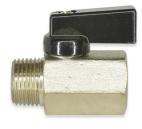
This is a Chrome-plated Forged Brass Mini Ball Valve with a Chrome-plated Brass ball. The maximum working pressure is 450 psi, 142 psi at 356°F, and 355 psi at 212°F. Available in female by female and male by female. Available with a flag handle, a lever handle, or a tee handle, or can be adjusted with a screwdriver.
