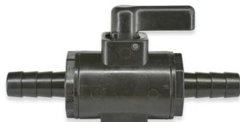
The PJV Series Micro Ball Valves are of Polypropylene and reinforced fiberglass with a 90-degree rotating handle and FKM O-rings. The standard pressure is 150 psi with a maximum temperature of 150° with a maximum pressure of 300 psi at 70° F.
