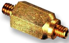
The CLCV Series Brass Check Valves have 10-32 inch ports, a Nitrile seal, and a Stainless Steel spring. It permits flow in only one direction and is used for air and hydraulics. The input psi is 300 maximum. The crack pressure is 1/2 psi and the temperature range is 32° F to 230° F. The 1/8-inch valve has a maximum input pressure of 1000 psi. Otherwise, all other attributes are the same as the 10-32 inch valve.
