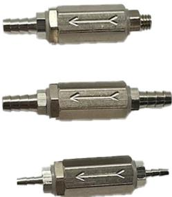
The BPCV Series Brass Piston Check Valves with nickel plate, are available with 10/32 Female UNF threads. Added to this main configuration is male 10/32 fittings or 1/16, 1/8, 3/32, inch barbs added.
