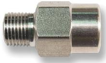
The PSCV Series Brass or Stainless Steel Piston Check Valves ensures a positive bubble-tight seal. They have a cracking pressure of 1 psi, a maximum pressure of 500 psi, and a maximum working temperature of 250° F. The standard unit is Brass with a 302 Stainless Steel spring and Steel retainer. Optional springs of 3, 5, 9, 15, 20, 25 psi. Also available in a 316 Stainless Steel body (shown) with a Hastelloy® spring. 1, 3, 15, and 25 psi. Seals available are Buna, EPDM, or FKM.
